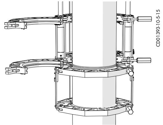
Support the carriage and loosen the clamp knobs on the fixed jaws and open the jaws.
