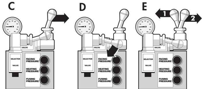
Allow joint to cool under pressure according to pipe manufacturer's or appropriate joining standard's recommendations.
