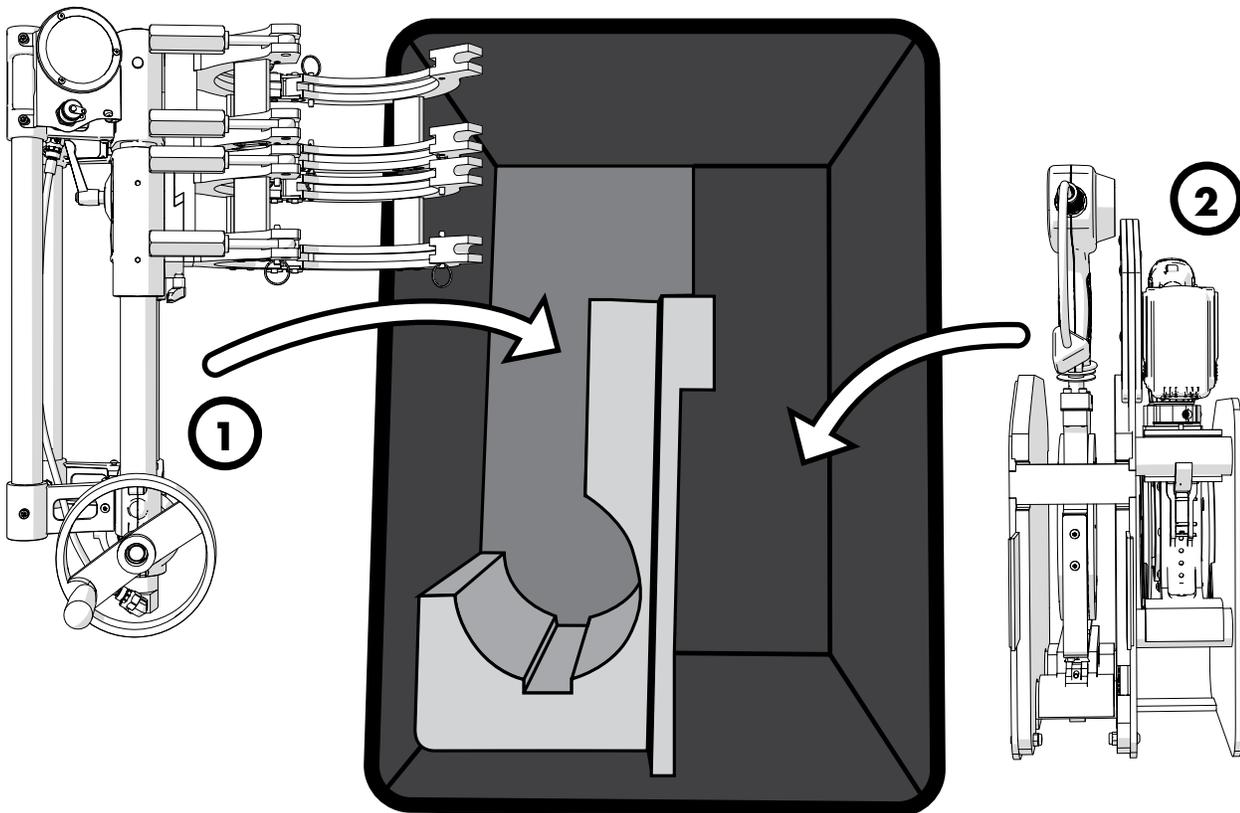
There are two socket fusion jaw foams that can be removed to store the socket fusion jaws.
