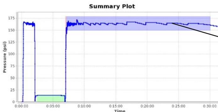
Pipe is cooled at fusion pressure for recommended cooling time.
