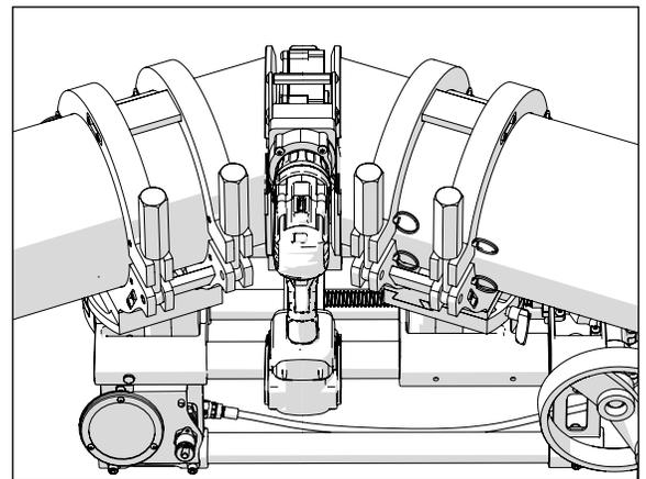
If the facer stalls, reduce the amount of pressure applied with the handle until it begins to cut again.
