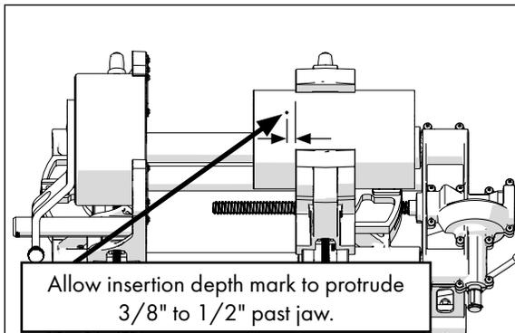
Allow insertion depth mark to protrude  $3/8$ " to  $1/2$ " past jaw.
