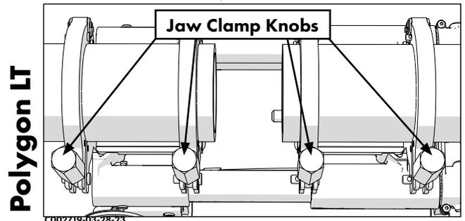
The clamp knobs are equipped with a ball thrust bearing, which permit the operator to develop high clamp forces with minimal effort.
