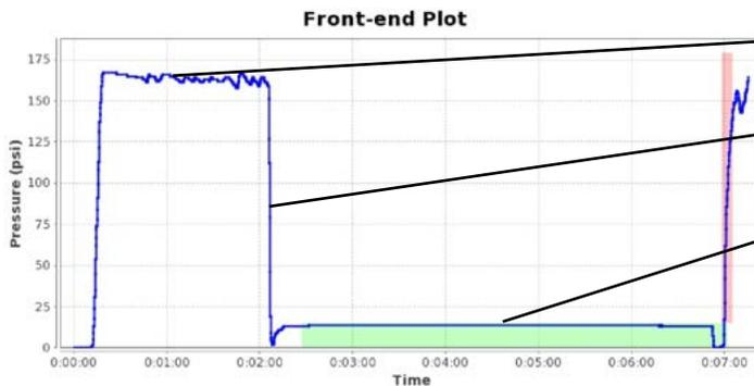
Bead up at recommended fusion pressure applied from the handwheel.
