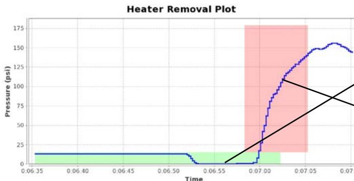
Carriage is opened and heater is removed.
