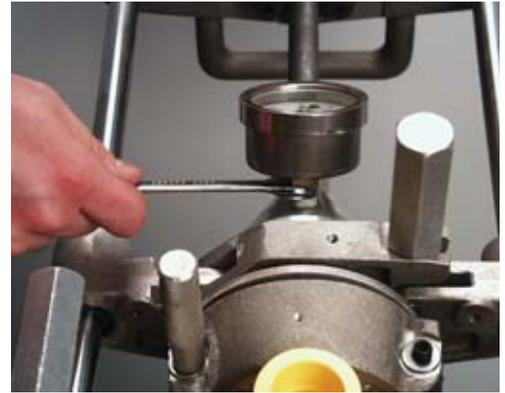
Add or remove hydraulic fluid until the level is approximately 1/2" from the top of the port.
