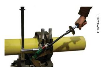
wrench adapter (Part # 713901). Using a torque wrench of a different length will result in different forces from the torque
