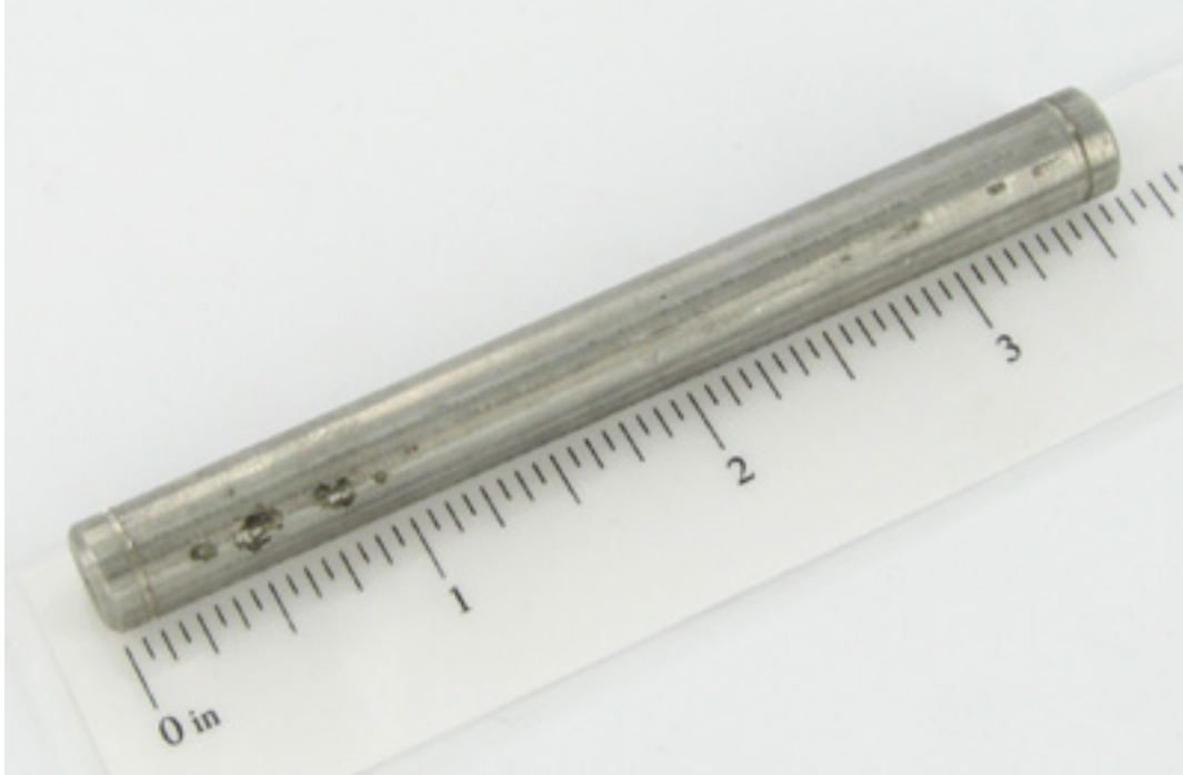
1ips trigger&body pivot pin
