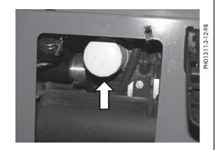
The oil drain plug is located on the bottom of the oil pan.
