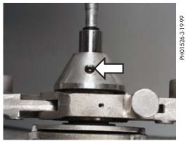
Reinstall gauge with Teflon tape applied to threads. Check to see if the needle indicates pressure as the gauge is being screwed on. If so, remove the gauge and use a clean rag to remove some hydraulic fluid. Repeat until no pressure is indicated while screwing gauge on.
