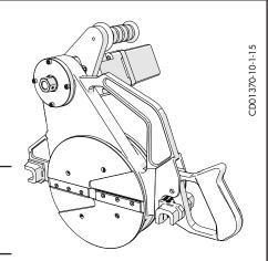
The facer has a handle that latches into place on a guide rod. The handle must be pulled out to unlatch and remove facer.
