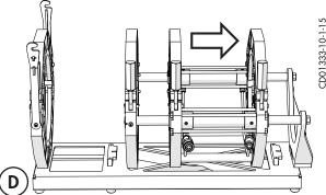
E) The 3-Jaw carriage is ready to be used for fusion.
