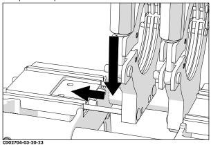
6) Slide the other jaw over the pins on the outer jaw side of the jaw base plate.
