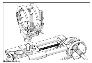
4) Install the other set of jaws in reverse order. Install the movable jaw first and then open the carriage so that the fixed jaw can be installed. Tighten both clamps after installation to secure the jaws in the Polygon™ base.
