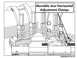
Ensure any gap between the pipe ends is within the limits of the fusion procedure being used. If not acceptable, reinsert facer and reface.
