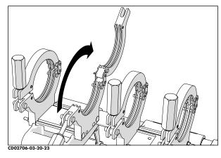
2) Remove the quick release pins from the upper and lower jaws.
