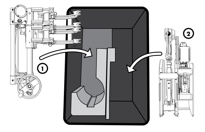
There are two socket fusion jaw foams that can be removed to store the socket fusion jaws.
