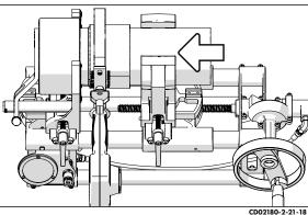
Heating time starts when the pipe and fitting are fully inserted onto the heater adapters.
