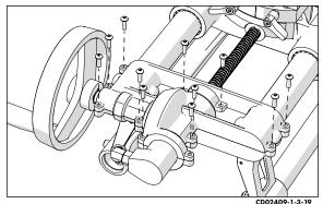
2) Lift off the top cover and drain the oil into a clean drip pan.
