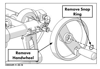
2) Remove the handwheel from the shaft.
