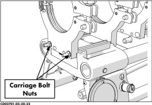
2) Slide off the outer jaw from the jaw base plate.
