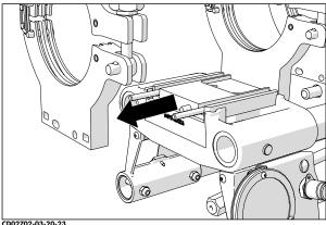
3) Slide off the inner jaw and carriage bolts from the jaw base plate.
