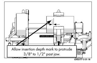
5) Open the jaws enough to allow the heater to be inserted.
