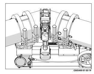
If the facer stalls, reduce the amount of pressure applied with the handle until it begins to cut again.
