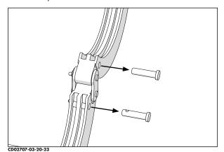
3) Install the appropriate sized inserts into the lower and upper jaws of the machine.
