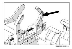
**3)** Loosen the back up bar and position the bar against the fitting. The back up bar can be removed and turned around to an alternate position in case the bar doesn't fit against the fitting properly.
