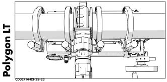
**4)** Tighten the clamp knobs on the outside jaws to prevent pipe from slipping. Hand tighten the inside clamp knobs to allow for HI/LO adjustment. Remove the facer.
