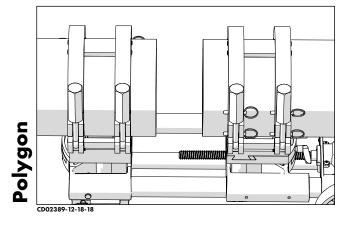
5) Tighten the clamp knobs on the outside jaws to prevent pipe from slipping. Hand tighten the inside clamp knobs to allow for HI/LO adjustment.
