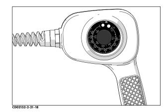
The heater has a green indicator light which will flash on and off. This indicates that the controller is operating normally. If the green indicator is not flashing then the controller may not be operating properly. If this occurs, disconnect power and have the heater repaired by a McElroy Authorized Service Center.
