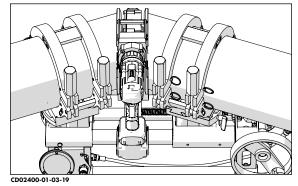
6) Clamp the jaws by inserting the handle into the pit of the jaw, and rotating the handle up toward the jaw. If there is no tension during clamping, open the handle and rotate the tension knob then try to clamp again. Repeat this until the jaw clamps firmly on the pipe. Bring the pipe ends together under pressure to ensure there is no slippage.
