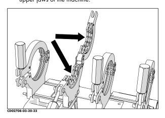
4) Install the quick release pins into the jaws to retain the inserts.
