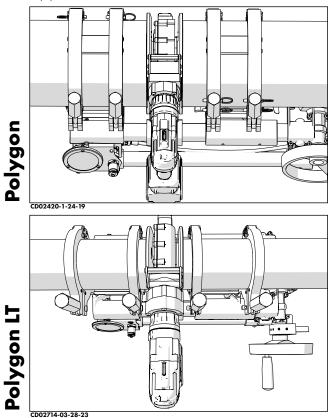
If the facer stalls, reduce the amount of pressure applied with the handwheel until it begins to cut again.
