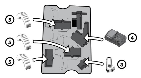
Insert with Socket Fusion Jaw Foam
