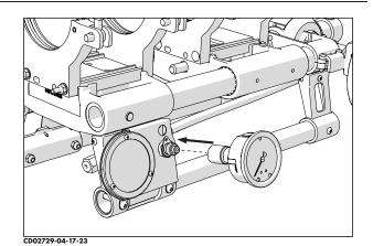
NOTICE: Do not pressure the machine greater than 100 PSI. Over-pressuring the gauge will damage the gauge and will no longer read pressure correctly.
