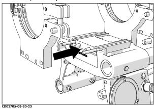
7) Install the two nuts on the carriage bolts and tighten to secure the jaws to the jaw base plate.
