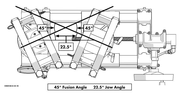
The mitered fusion angle is set by loosening the jaws rotation and rotating the jaws to the desired angle using the angle scale gauge.
