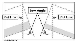
4) Set the desired fusion angle. Each jaw will need to be adjusted to set the correct jaw angle based on the fusion angle. Refer to section "Mitered Fusion Angles" for instructions on how to set the jaw angles.
