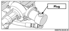
**3)** Loosen the plug on the tee fitting behind the pressure gauge.
